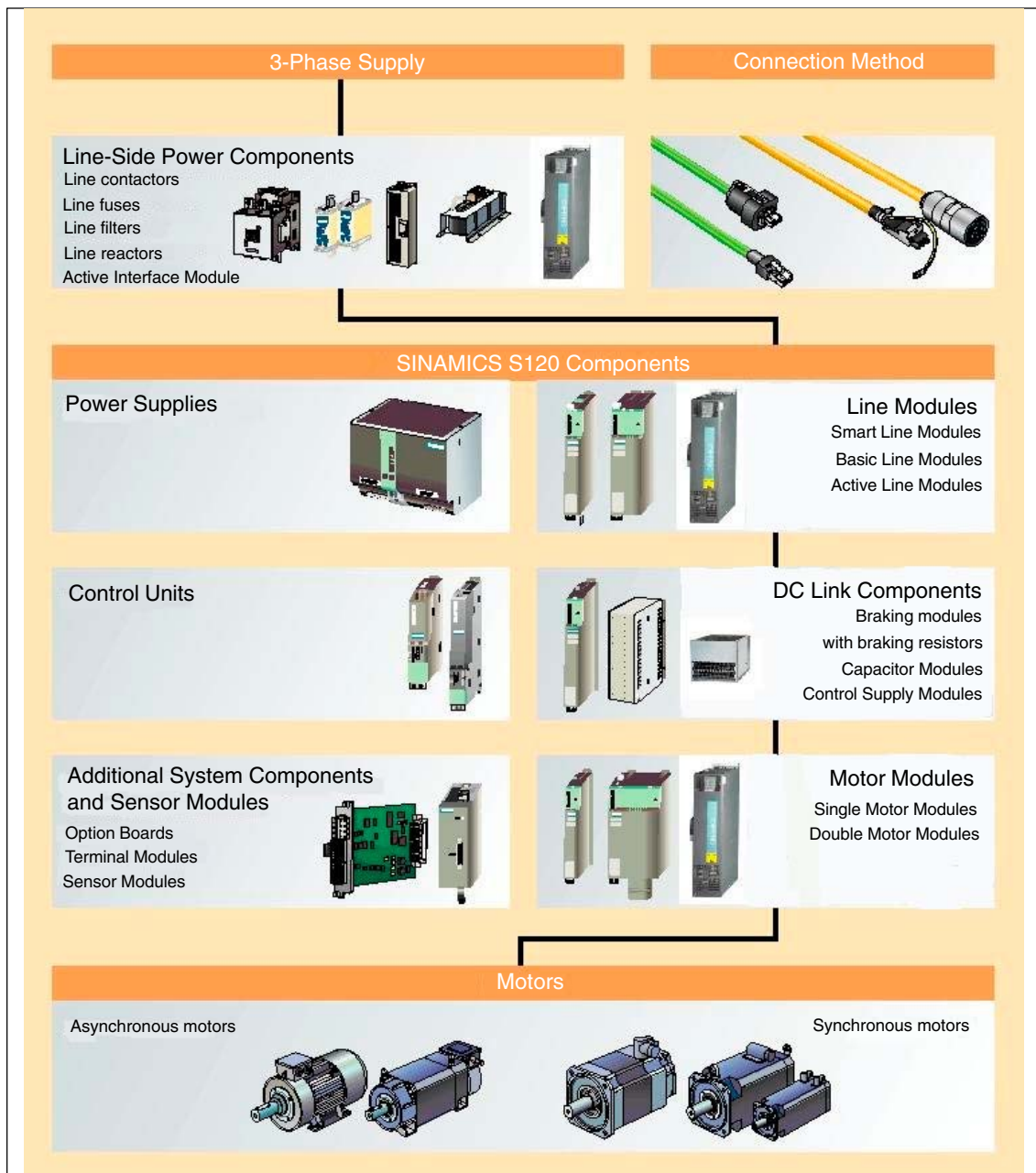
Fig. 1-7 SINAMICS S120 component overview
